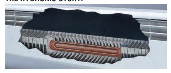
The electric heating element is partially submerged in an inert heat transfer fluid totally sealed in a large 7/8" diameter copper tube spanning the length of the heater. This thermal mass transfers heat evenly across the entire length of the heater. The HBB series provides uniform warmth with longer heat retention and minimal temperature variation.
